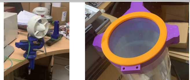
Current developments: 3D printed thruster and front end-cap
