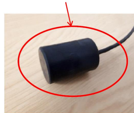
Potted modem (42mm diameter by 60mm long)
