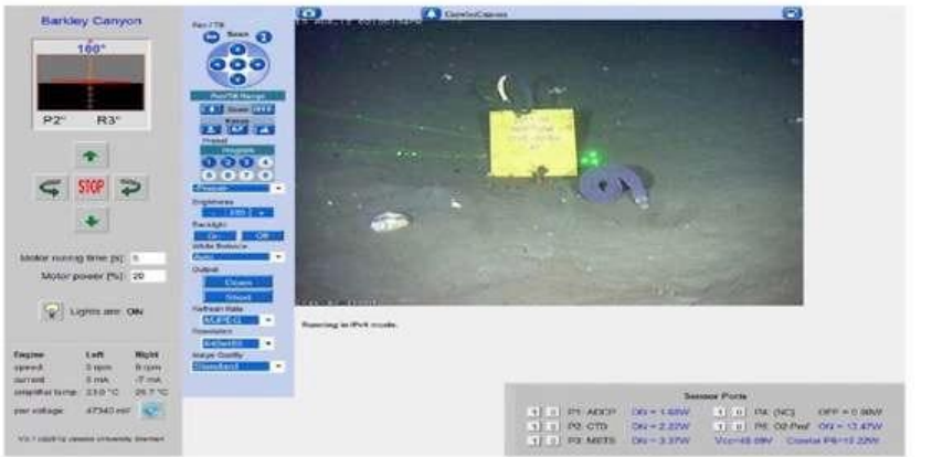
Fig. 4. Screenshot of the Crawler control window, incorporating both Crawler and camera movement options bars, and sensor port output bar. The sizing laser is also activated. One of the yellow navigation markers placed on the seabed by an ROV during Crawler installation is evident. (For interpretation of the references to colour in this figure legend, the reader is referred to the web version of this article.)
